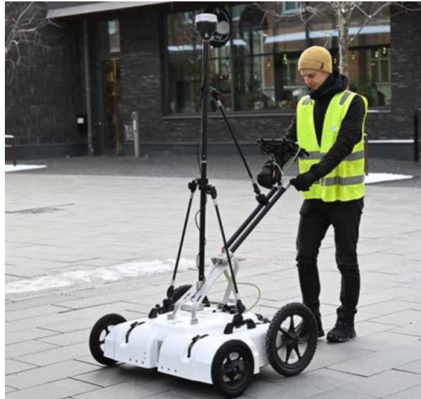
Figure 2: Push Cart System for areas inaccessible to vehicles
