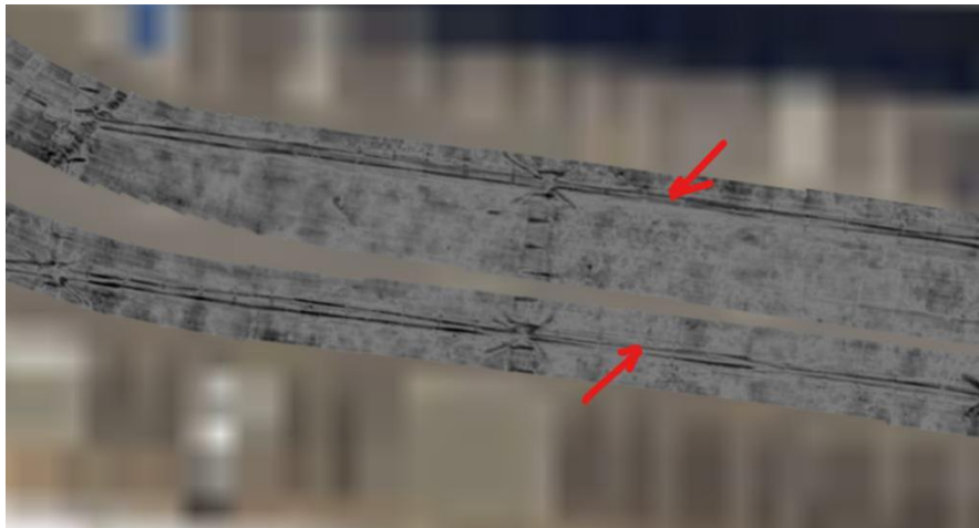
Figure 5: Condor software visualisation of old gantry rails below the asphalt layer
