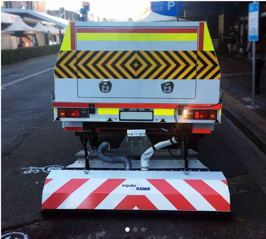
Figure 1: Mobile system with Raptor GPR mounted to the rear of a survey vehicle.
